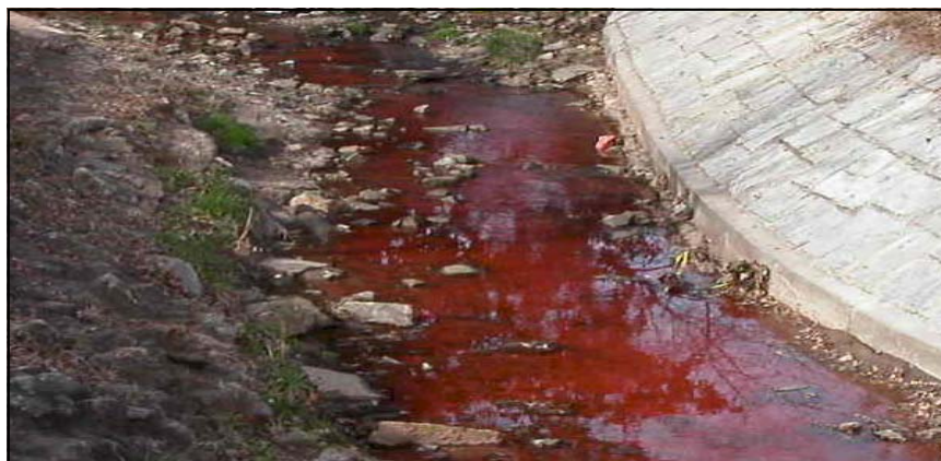
Tanyard Creek resembled the Nile River when it turned red in biblical times, but tracer dye caused this creek to flow red.
